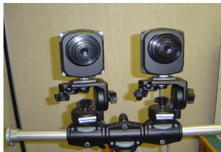
Figure 5.1: The stereo rig; a close up of the dual IR cameras mounted on a tripod.
