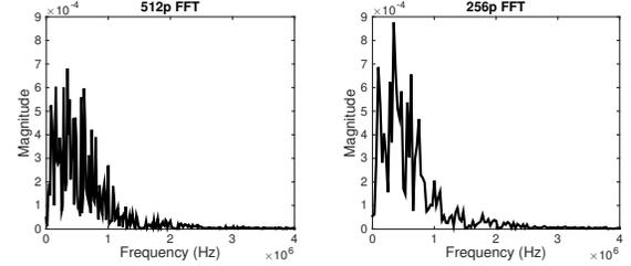
Fig. 6. FFT PSDs (8Ms/s) with different number of FFT points.
