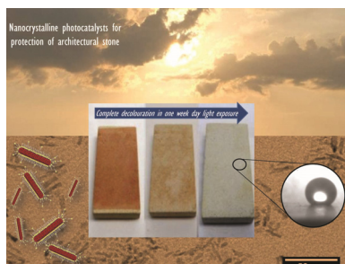
Figure 1: Bleaching of Methyl Red dye on PL surface treated with TiO 2 NR after 1 week exposure to day light. Inset: Water contact angle highlight the hydrophobicity of the treated surface.
