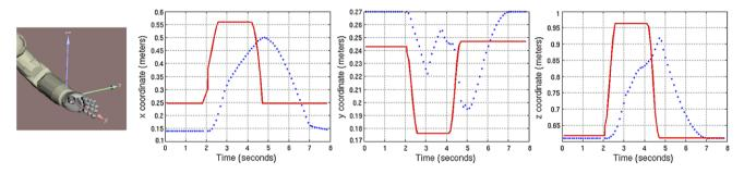
Fig. 8 Plots of x-, y- and z-coordinate respectively of the wrist positions of the ACE body model (*solid*) and the physical robot (*dotted*) during gesture execution [36]
