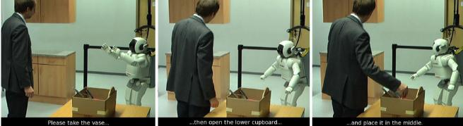
Fig. 12 Example of a multimodal three-chunk utterance delivered by the robot during interaction. Three different types of gesture are used (left to right): iconic gesture illustrating the shape of the vase;
