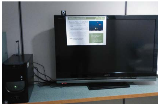
Figure 3. Feedback device (PC and computer display) and camera and microphone for data collection.
