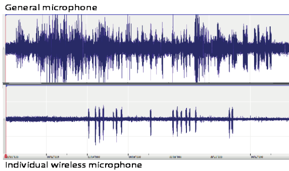
Figure 2. Selectivity of the wireless microphone. Upper trace: recording of 6 animals in an aviary using a standard microphone. The wireless microphone (lower trace) records the vocalizations of one animal only. This allows the correlation of individual vocalization patterns to describe the vocal interactions within this group.
