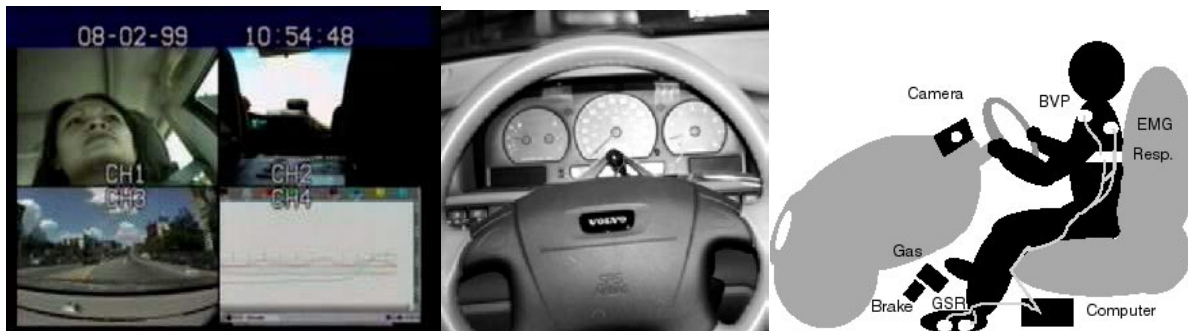
Figure 2. Driving offers a situation where emotions can be monitored using a driver facing camera (shown in the center) and multiple external cameras (captured video shown left) and where physiological signals can be captured by a computer (right) where many emotions are strongly felt, especially frustration, anger, and “stress” during traffic. Occasionally, emotions such as sadness or joy may occur in response to music on the radio. Driving is real life, unexpected things do occur and your life is really on the line. The driving environment offers a compromise between laboratory studies with high internal validity but limited stimuli and fully ambulatory with high external validity but difficult to interpret data.
