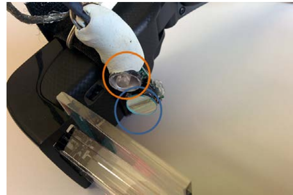
Figure 2. Red circle marks infrared led. Blue circle marks cold mirror in front of the camera lens.
