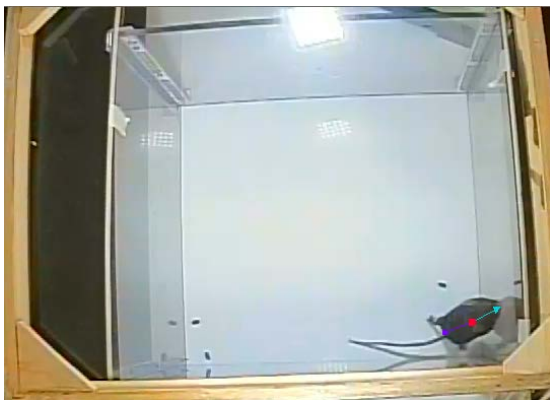
Figure 3. Automated mouse tracking in Ethovision 10.0. Mouse center, nose and tail points are tracked to determine velocity and total distance travelled.
