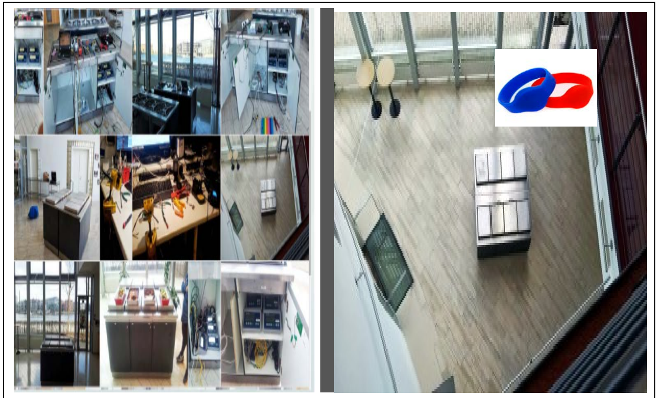
Figure 1. The Intelligent Buffet. To the left an overhead picture of the IB in the eat area of the FoodScape Lab. The left of the picture illustrates how the electronics is covered by the body of the buffet. The picture to the right shows the IB from the position of the overhead cameras. On the top right corner the picture shows inserted the wrist bands based on Near Field Communication technology that allows for distinguishing between the subjects taken food from the buffet. The wrist bands communicate with a receiver on the side of the buffet under each scale.
