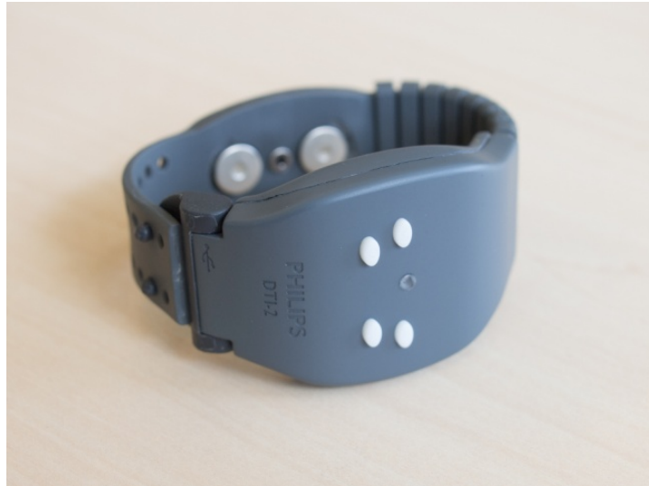
Photo 1. The Digital Tension Indicator – 2 (DTI-2) used in the current study to assess the skin conductance level of the participating patients.
