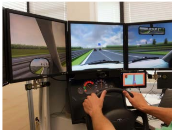
Figure 1. Driving simulator setup. The driving scenario is shown on an array of five LCD screens (of which only the middle three are shown). A sixth screen below the middle screen shows the standard dashboard display with speedometer and RPM display. A small screen (18 cm diagonal), mimicking a display in the mid console, is attached to the right of the sixth screen to present the displays under investigation.
