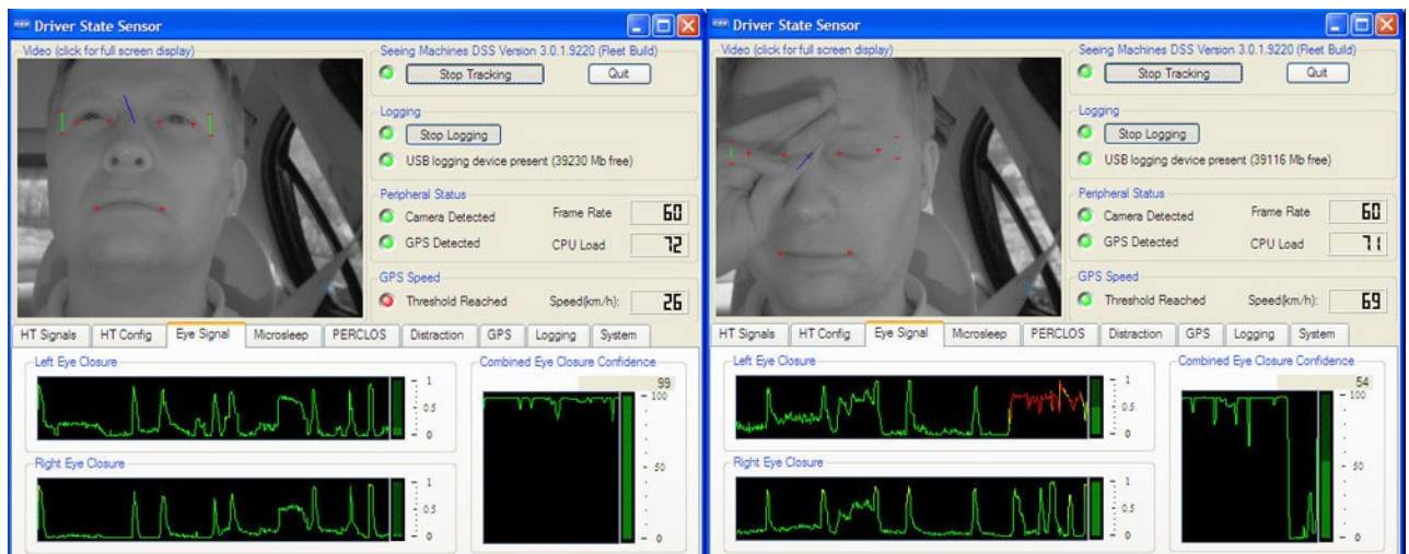
Figure 5: Driver State Sensor (DSS) device developed by SeeingMachines [62].
