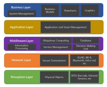
Figure 1. Layered architecture of IoT [14], Adapted.
