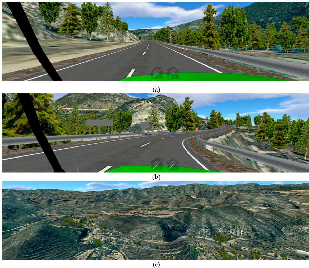
Figure 5. Captured images from a multilayer-based edited driving scenario methodology: (a) Driver's view along a straight road section; (b) Driver's view along a curve road section; (c) Aerial view of a section of the road [44].
