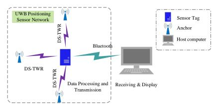
Figure 4. Schematic diagram of ultra-wide band (UWB) positioning system.
