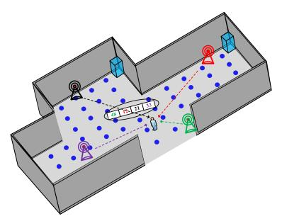
Figure 1. The fundamentals of WiFi fingerprinting indoor localization.
