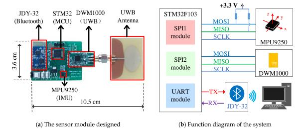
Figure 7. The UWB-IMU sensor module.
