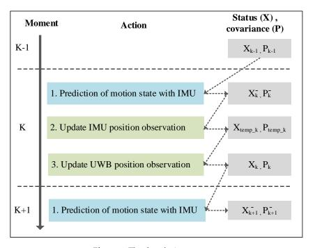
Figure 6. The data fusion process.
