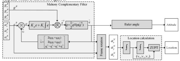
**Figure 5.** Schematic diagram of the inertial measurement units (IMU) attitude and position estimation. ZUPT: zero velocity update.
