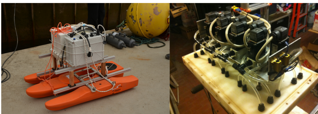
Figure 8. Towed trimaran equipped with an Autonomous Water Sampler (AWS).
