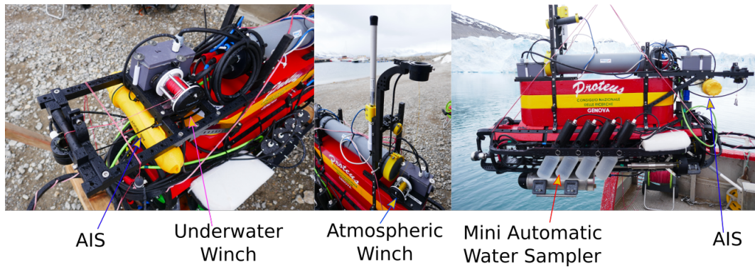
Figure 24. The integration winches and Mini Automatic Water Sampler (MAWS) on-board PROTEUS.
