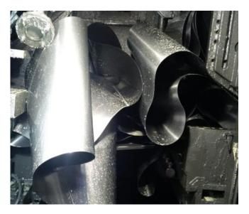
Figure 2. Consequences of strip rupture in the cold-rolling process.
