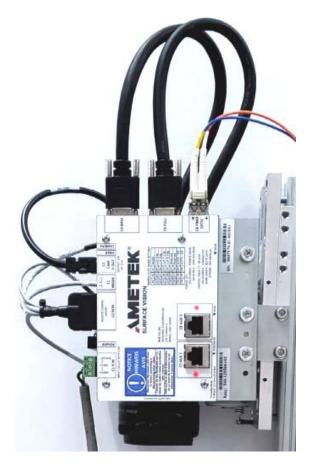
Figure 4. Surface inspection camera with Ametek Camera Link Interface module [31].
