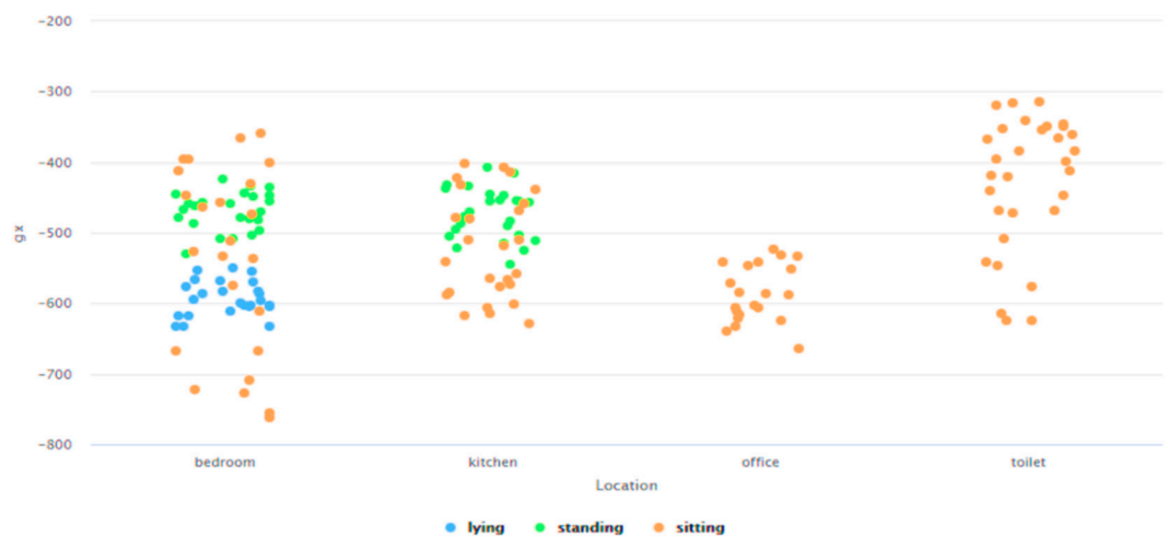
Figure 23. Analysis of the gyroscope data (in the X-direction) for different behavioral patterns associated with different ADLs performed in the given simulated smart home environment.
