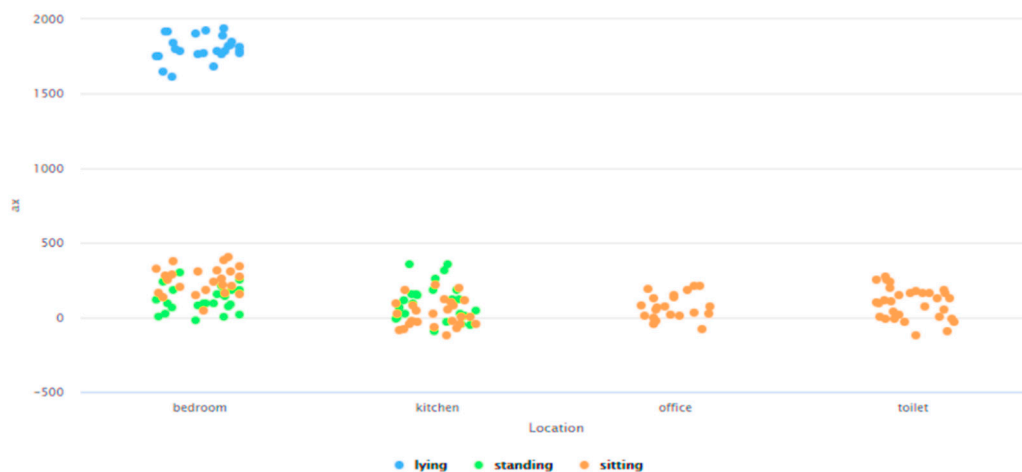
Figure 20. Analysis of the accelerometer data (in the X-direction) for different behavioral patterns associated with different ADLs performed in the given simulated smart home environment.
