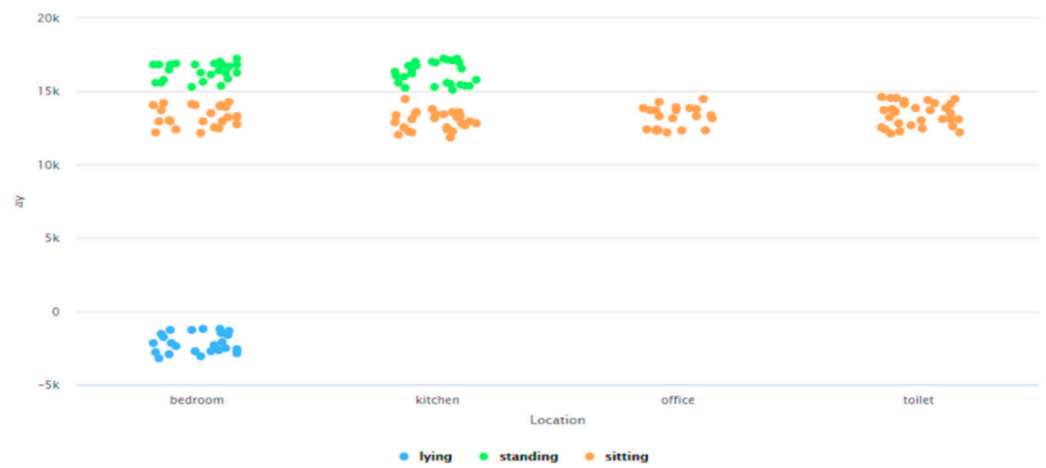
Figure 21. Analysis of the accelerometer data (in the Y-direction) for different behavioral patterns associated with different ADLs performed in the given simulated smart home environment.
