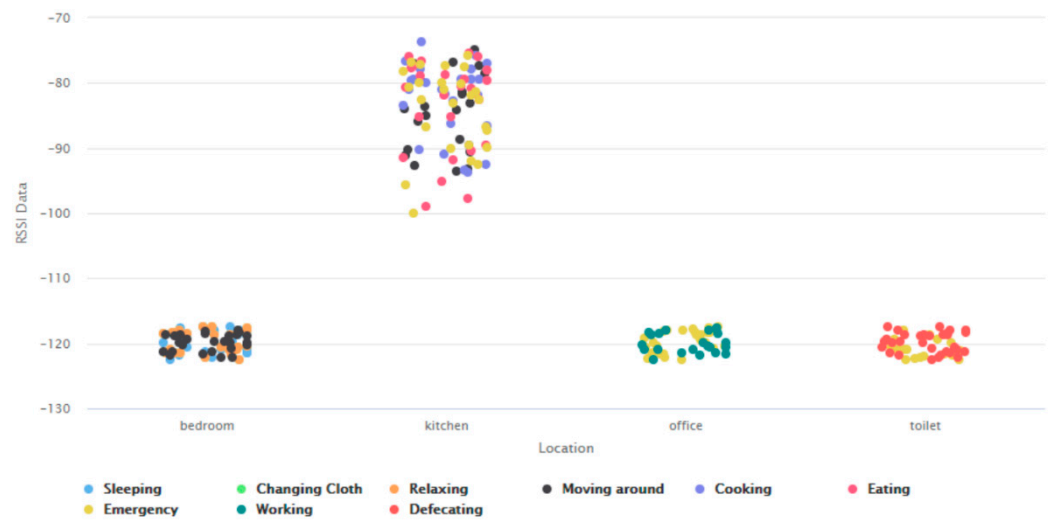
Figure 14. Analysis of RSSI data coming from different BLE scanners and BLE beacons when different activities were performed in the kitchen.
