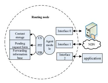
Figure 4. Relationship between NDN routers and proxy servers and applications.
