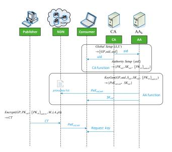
Figure 1. Flow of the Named Data Network (NDN) access control system.
