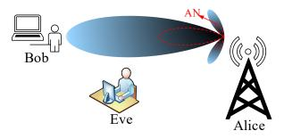
Figure 13. Secrecy beamforming with artificial noise (AN).
