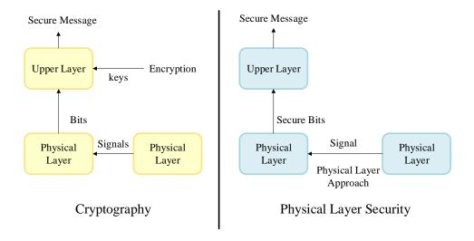
Figure 3. The difference between cryptography and physical layer security approaches [28].
