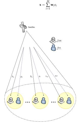
Figure 22. Multi-beam satellite communication network [114].
