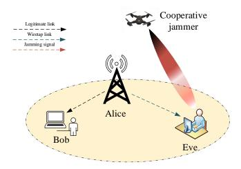
Figure 18. Cooperative jamming using unmanned aerial vehicle (UAV).
