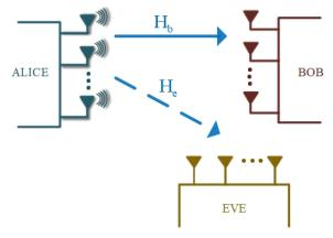
Figure 9. MIMO wiretap channel model [29].
