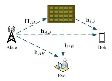
Figure 19. Intelligent Reflecting Surface (IRS) system model [14].
