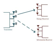
Figure 17. A multiple-input multiple-output (MIMO) system for Simultaneous Wireless Information and Power Transfer (SWIPT).
