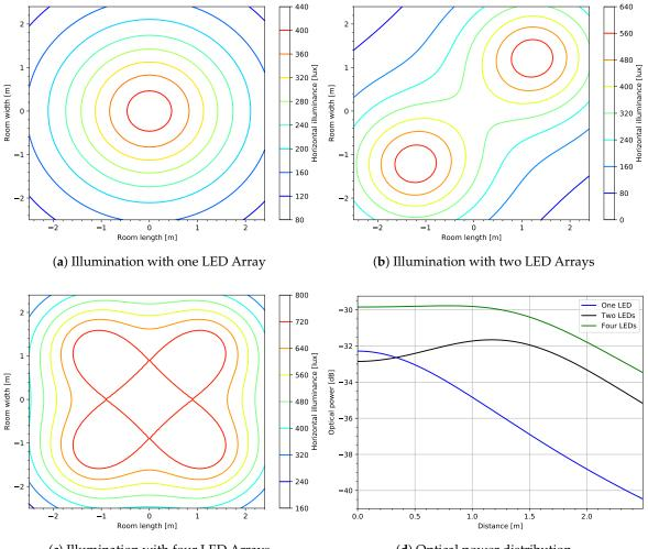
(c) Illumination with four LED Arrays
