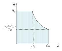
Figure 8. Wyner's transmission rate vs equivocation rate.
