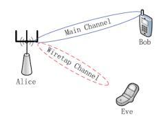
Figure 4. Physical layer security (PLS) system model.
