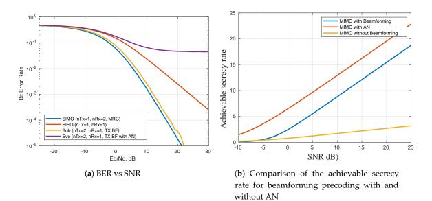
**Figure 16.** Bit error rate (BER) and secrecy rate performance metrics simulations for different precoding schemes.
