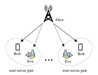
Figure 12. System model of multi-user and eavesdropper pairs with beamforming.
