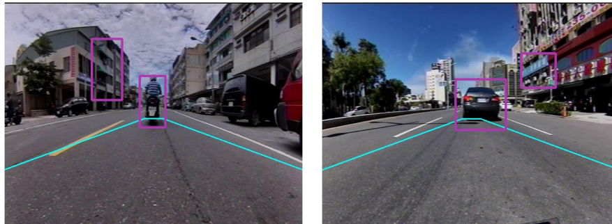
Figure 17. Error detection of the Haar-like algorithm.
