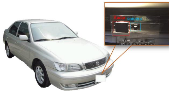
Figure 11. Experimental car and sensors setup.
