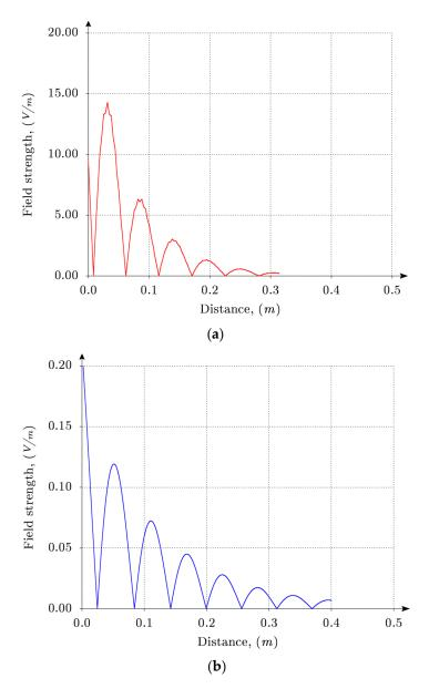
**Figure 15.** The distribution of the electric field component of the EM waves propagating along the surface at the frequency f = 2.45 GHz: the creeping wave (**a**); the surface wave (**b**).
