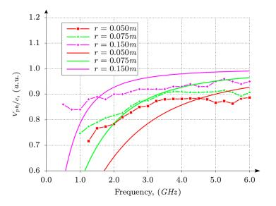
The frequency dependence of the normalized phase velocity of the CW using Equation (17) is presented in Figure 18 together with full-wave simulation results.
