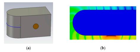
**Figure 14.** The model used for the surface and creeping wave simulation: (**a**) front sight; (**b**) the electric field distribution (top view).
