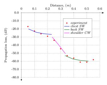
**Figure 21.** Measured insertion loss between the antennas along the path on a body. The distance between the antennas is shown on the horizontal axis, and the insertion propagation loss is shown on the vertical axis. Red dots represent the measured receiving antenna positions. The blue and green line is the predicted SW propagation loss from the modeling results presented in Figure 15a, and the magenta line is the predicted CW propagation loss from the modeling results presented in Figure 15b.
