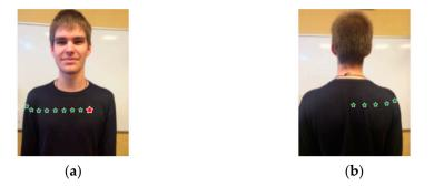
**Figure 19.** (**a**)The antenna position over the human body. (**b**)The position of the stationary transmitting antenna is shown by the red star; the green stars show the receiving antenna positions.
