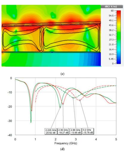
**Figure 12.** (a) Electric field distribution in the finger excited by the printed antenna: printed antenna placed on top of the finger, (b) electric field distribution inside the modeled tissues at 750 MHz and (c) at 2225 MHz; (d) return loss of the antenna: red curves—diseased bone, green curves—healthy bone, solid lines—modeling, and dashed lines—experiment [42,43].
