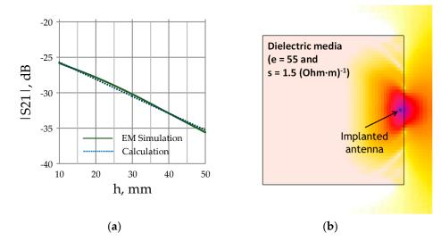
**Figure 6.** (a) Transmission coefficient module  $|S_{21}|$  versus distance between the implanted dipole and the dielectric medium surface *h*. (b)The electric field distribution radiated by an antenna inside the dielectric medium.
