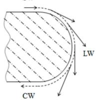
Figure 13. Types of waves on the surface of a complex shape.
