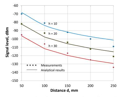
**Figure 7.** Measured signal power level versus distance *d* between the reader antenna and the box with the tissue-equivalent liquid for different values of distance *h* between the implanted dipole and the tissue surface. The results of calculation by (8)–(10), taking into account the path loss and medium mismatching, are shown by solid lines, and the dots present the measured results.
