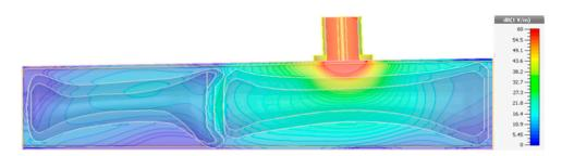
Figure 11. Electric field distribution within the finger volume excited by the open-end coaxial probe.
