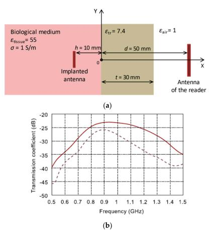
**Figure 8.** (a) A scheme of the structure containing the implanted antenna with matching layer placed between the biological tissue and the reader antenna; (b) the transmission coefficient between the antennas: Transmission coefficient is shown by the solid line for the structure with matching layer and by the dashed line without it.
