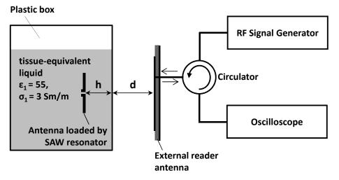
**Figure 4.** The scheme of the experimental setup for measurement of the transmission coefficient of the wave propagating through the interface.
