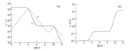
**Figure 2.** Frequency dependence of the real and imaginary parts of the relative dielectric permittivity (**a**) and conductivity (**b**) of biological tissue with averaged parameters calculated by the Debye formula.
