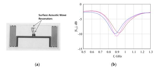
**Figure 5.** (a) The design of the implanted dipole loaded by SAW resonator; (b)return loss measured for three test samples of the implanted dipole in the tissue-equivalent liquid.
