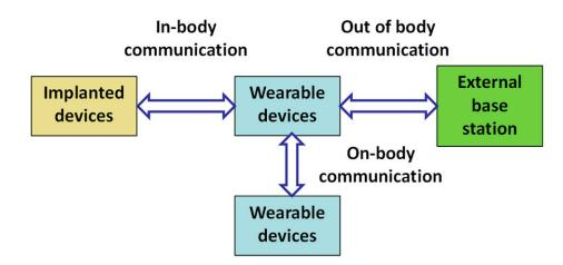
**Figure 1.** The system for collecting and transmitting information about the state of the human body. The system includes implanted and wearable devices and an external base station receiving collected information.
