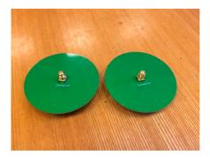
Figure 20. Two manufactured disc antennas used for on-body propagation loss measurements.
