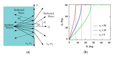
**Figure 3.** The spherical wave propagation across the interface between two dielectrics (**a**) and the dependence of the angle of refraction on the angle of incidence (**b**) for dielectrics with different values of permittivity ( $\varepsilon_1 = 55, 15, 5$ ) and  $\varepsilon_2 = 1$  [13,18].
