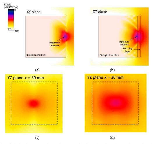
**Figure 9.** The E-field distribution: XY plane without (**a**) and with matching layer (**b**); YZ plane without (**c**) and with (**d**) matching layer.
