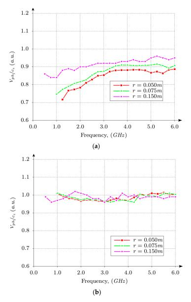
**Figure 16.** The normalized phase velocity of waves for different values of the phantom thickness: (a) creeping wave; (b) surface wave.
