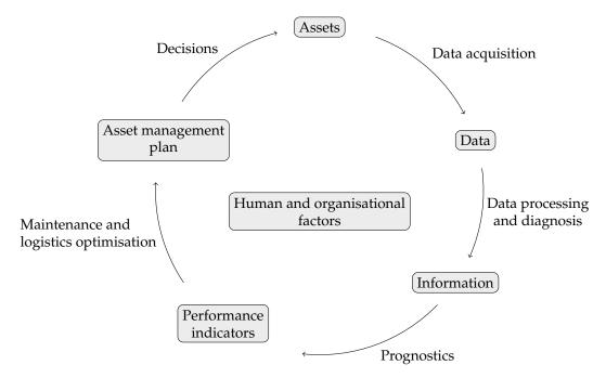
Figure 1. Predictive maintenance management process model.
