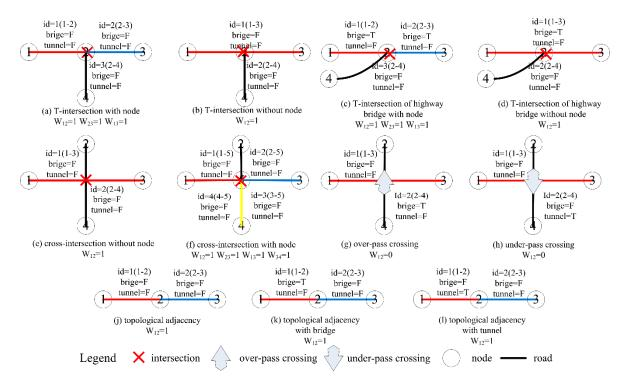
Figure 5. Typical topological and geometric relationships of road network.
