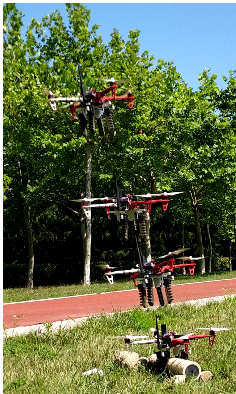
Figure 10. The proposed quadrotor helicopter system successfully landing on an outdoor non-flat surface with the support of the RBFNN controller.
