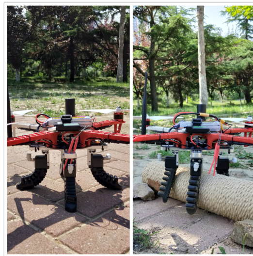
Figure 6. Quadrotor successfully landed on convex surfaces with the support of the proposed soft landing gear.
