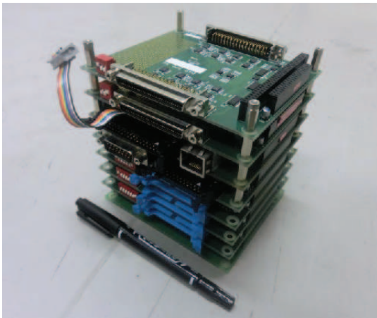
Figure 18: Photograph of TCU, which comprises a main FPGA board, 2 TPC-I/O boards, 3 PSA-I/O boards, a GPS-IO board, and a power board. Each board measures 100 mm × 120 mm.
