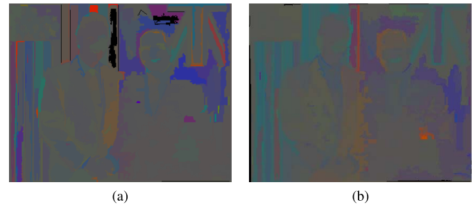
Fig. 17. IMs extracted from Figure 16. Successive JPEG compressions applied on the image, allied with a very low resolution, compromised the first step of the proposed method and leading our method to misclassify the image. (a) IIC. (b) GGE.
