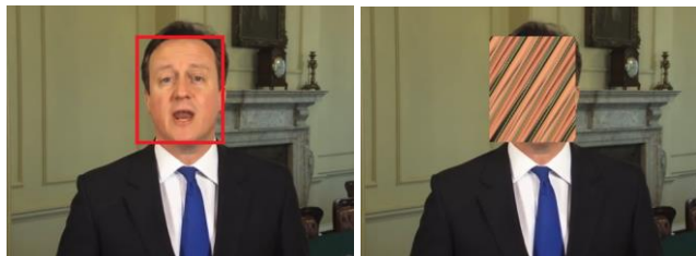
Fig.1. A detected face in video scrambled by using the Arnold transform.
