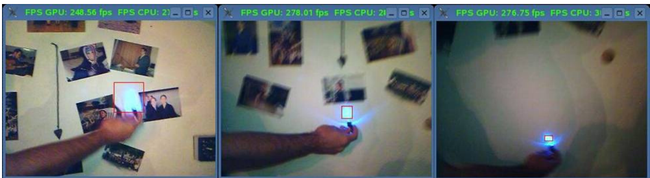
Figure 5.22: Tracking an LED light beam, with tracking algorithm's output shown as a red square.
