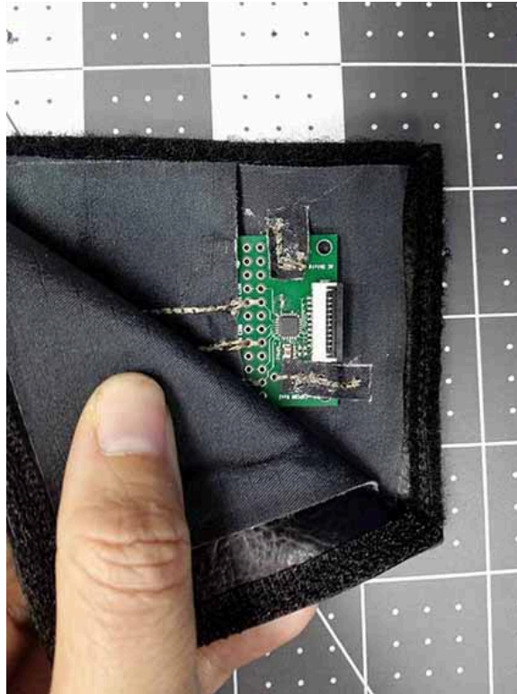
FIG. 5.5. Conductive threads connected to ground, shield and capacitive sensors connect to Capsense daughter board in the RestEaZe band.
