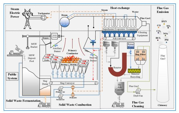
**Figure 4.** Process flow of an MSWI plant in Beijing. Note: Flue Gas1 denotes the flue gas at the furnace outlet. Flue Gas2 represents the flue gas at the inlet position of the induced draft fan. Flue Gas3 corresponds to the flue gas at the chimney outlet. Within the existing body of research, the predominant focus has been on Flue Gas1 and Flue Gas3.
