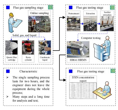
Figure 9. The detection process of DXN concentration [113].
