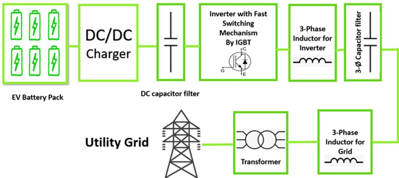
Figure 3. Fast bidirectional charger schematic for EV charging stations.
