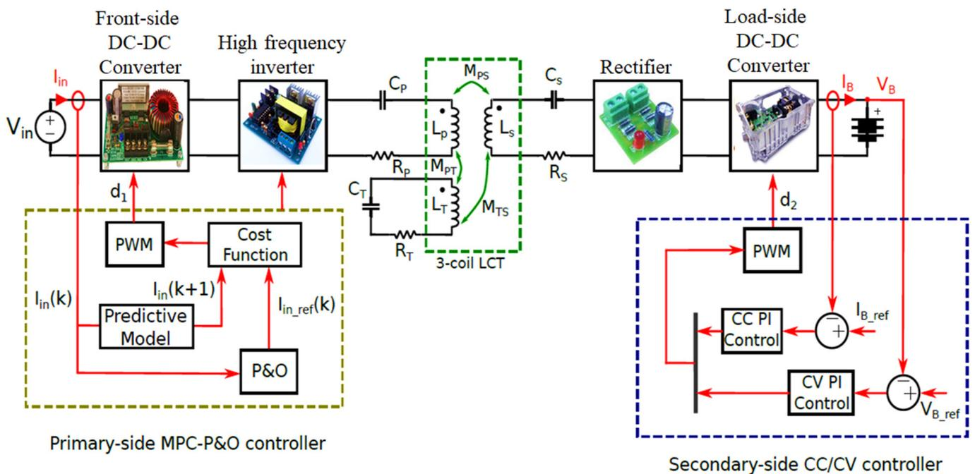
Figure 8. Control narrative in a wireless EV charger.
