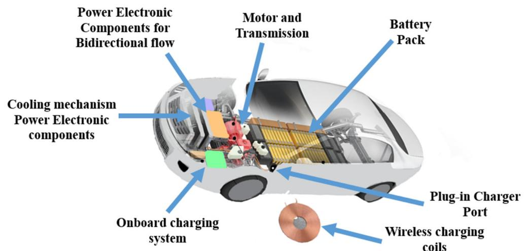
Figure 1. Conceptual EV structure and components.
