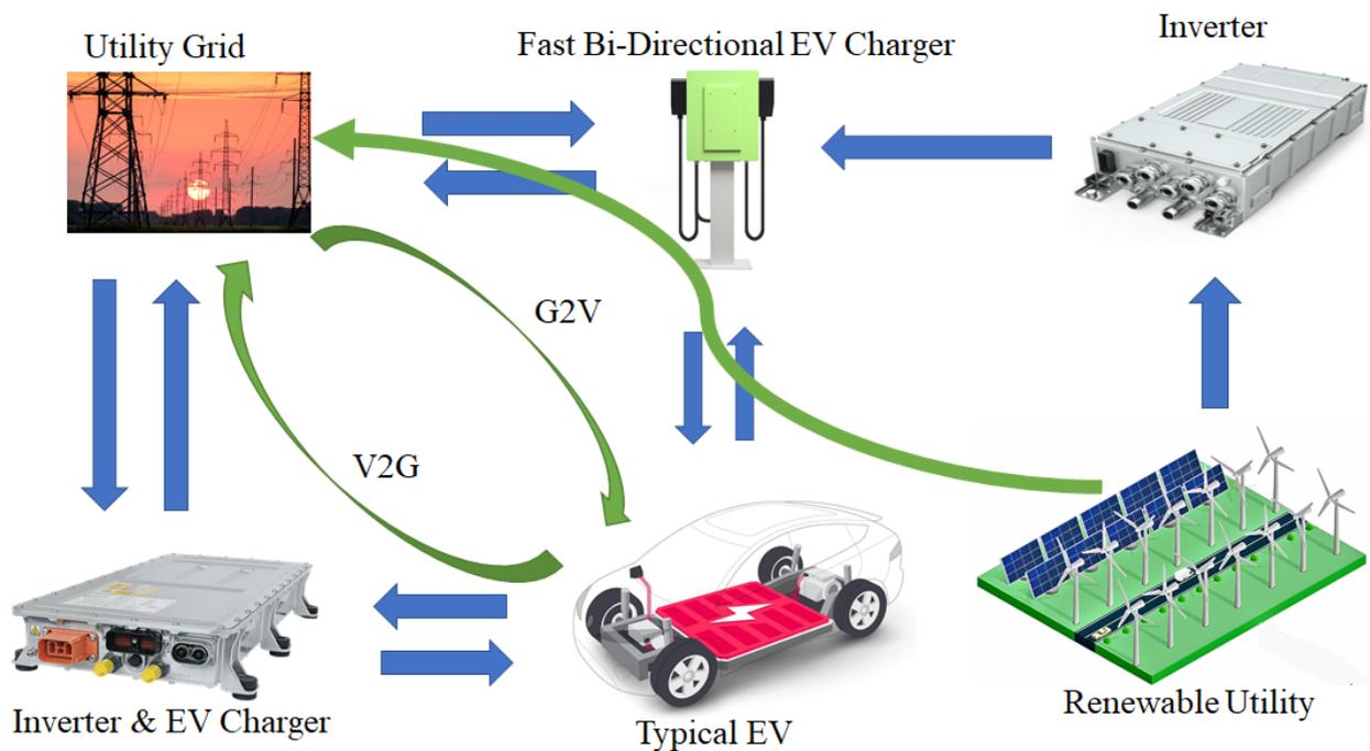
Figure 2. G2V and V2G power flows block diagram.
