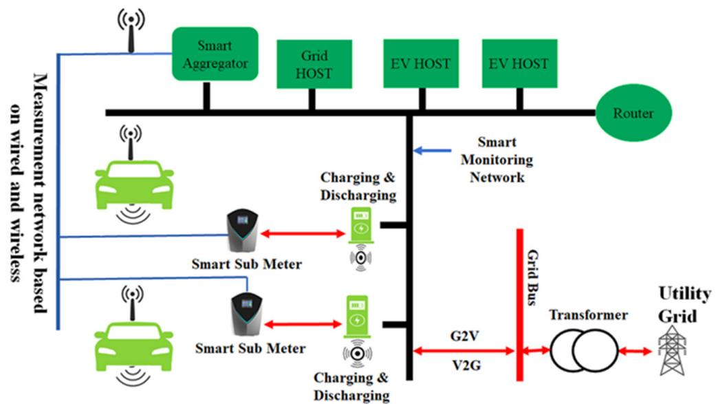
**Figure 6.** Smart meter architecture for bidirectional energy measurement on EV applications.
