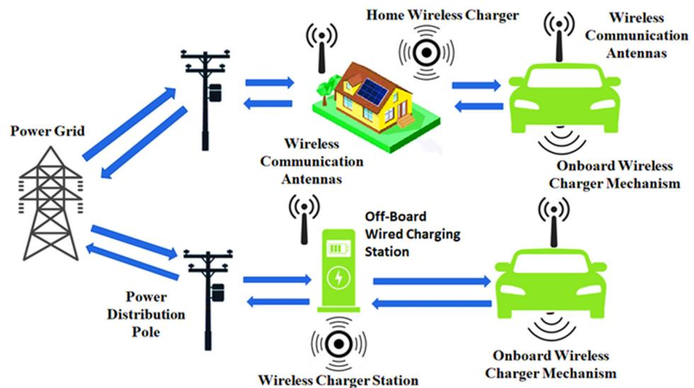
Figure 4. Power distribution line, plug-in, communication control links, and wireless charging technology with the grid.
