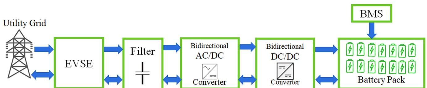
**Figure 5.** Uni-directional and bi-directional power flow for typical EVs.
