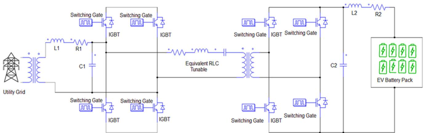
Figure 7. Bidirectional dual active full-bridge converter adoption.
