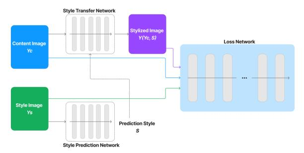
Figure 3. Overall network architecture.
