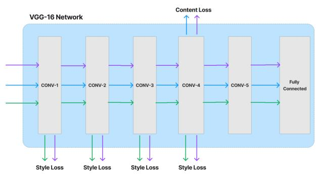
Figure 4. Loss network VGG-16.
