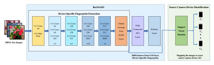
**Figure 2.** The hybrid ResNet–SVM to extract the new device-specific fingerprint without using PRNU to identify the source camera.
