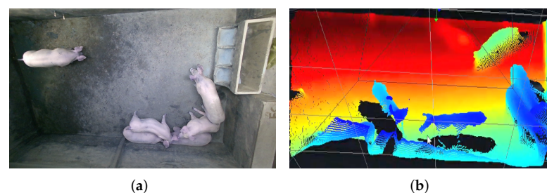
Figure 3. Camera top-view image and its corresponding 3D point cloud. (a) RGB image; (b) 3D point cloud.
