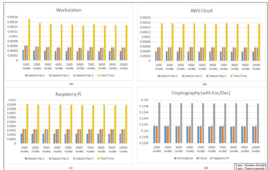
Figure 7. Performance with respect to the hash-chain fog/edge protocol total time on the (a) workstation, (b) AWS Cloud, and (c) Raspberry Pi and (d) for message exchange with cryptography.
