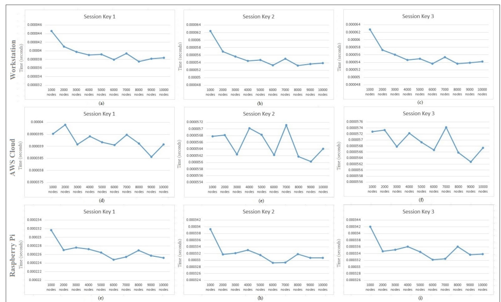
Figure 5. Session key generation time on the workstation for (a) Session Key 1, (b) Session Key 2, and (c) Session Key 3, the AWS Cloud for (d) Session Key 1, (e) Session Key 2, and (f) Session Key 3, and the Raspberry Pi (g) Session Key 1, (h) Session Key 2, and (i) Session Key 3.
