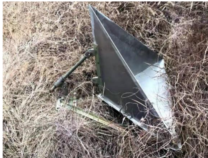
Figure 2. Triangular trihedral corner reflector used in the experiment.
