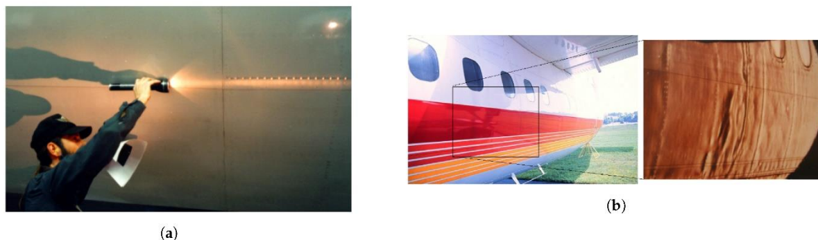
Figure 8. (a) An expert inspects the fuselage visually with a torch; (b) the fuselage picture is scanned, revealing surface micro perturbations produced by corrosion [16].
