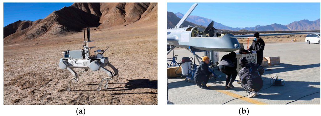
Figure 8. Field trial scene of UAV airborne NTN: (a) quadrupedal locomotion robot with Customer Premise Equipment (CPE) on board; (b) CH-4 UAV equipped with 5G base station and satellite antenna preparing to take off.
