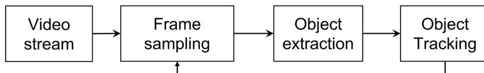
**Figure 13.** Overview of the object tracking method.
