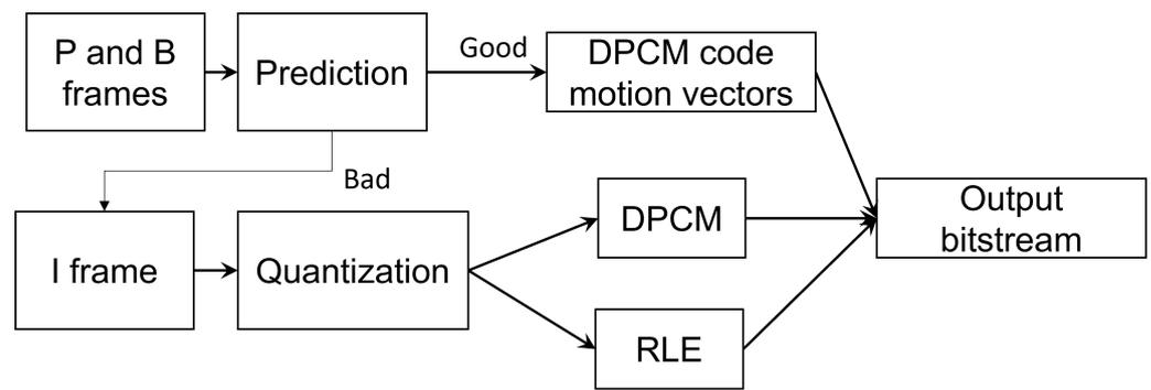
Figure 9. Flowchart of MPEG-1 encoding.
