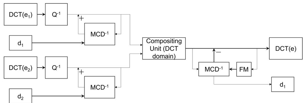
**Figure 10.** Compositing two DCT-based video sequences in DCT domain.
