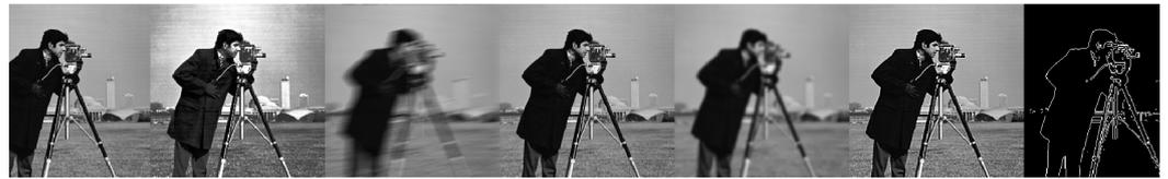
**Figure 2.** Output for different image enhancement methods. The operations applied, from left to right, are: original image, histogram equalization, motion blur, deblur using Wiener filter, smoothing with Gaussian filter, image sharpening, edge detection with Sobel operator.
