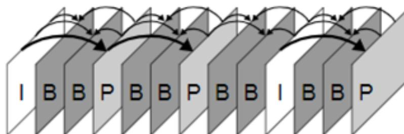
**Figure 8.** Intra (I) and inter (B and P) frames in a video sequence.
