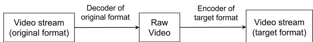
Figure 12. Conventional video transcoding flowchart.
