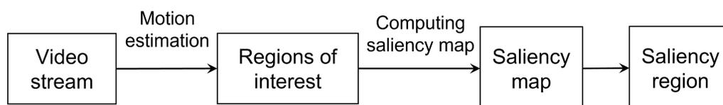
**Figure 14.** Flowchart for salient motion detection.
