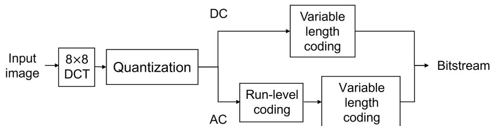
**Figure 1.** Flow chart for baseline JPEG for an image. An input image will go through multiple operations, including the discrete cosine transform (DCT), quantization, differential coding, and variable-length coding. The output is a bitstream with headers and markers containing side information for the decoder.
