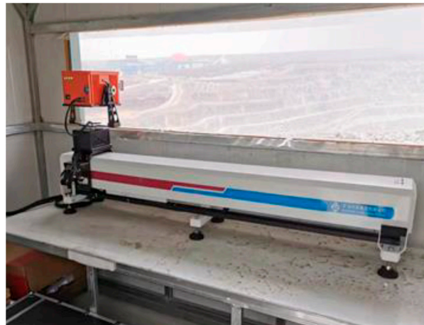
Figure 4. New FMCW-GBSA Radar developed by North China University of Technology in the quarry [63].
