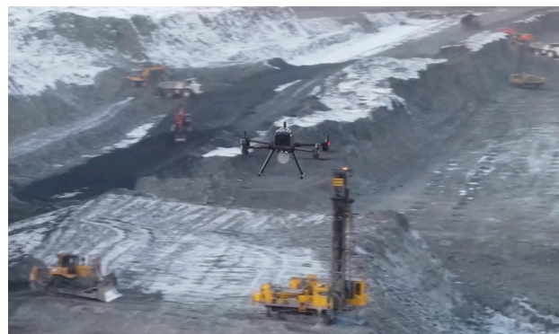
Figure 13. Preliminary control of drilling operations using the Matrice 300 Pro quadcopter (photo by authors).
