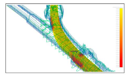
**Figure 11.** Three-dimensional model for the purpose of analysis of collision in underground mine workings possibility (Reprinted from Ref. [69]).
