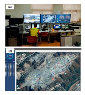
Figure 10. An open-pit mine in South Korea with a wireless communications system for fleet management of mine equipment. (a) Control center. (b) Main dashboard (Reprinted from Ref. [65]).
