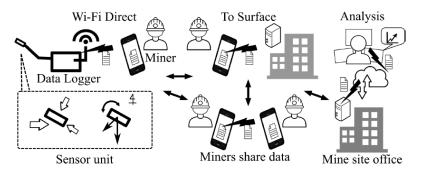
Figure 8. Design of the data transmission Wi-Fi monitoring system (Reprinted from Ref. [51]).
