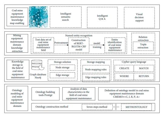
**Figure 5.** Architecture of the knowledge graph system for coal mine equipment maintenance (Reprinted from Ref. [42]).
