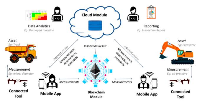
**Figure 13.** High-level architecture of Integrating the IoT and Blockchain Technology in the mine inspection (Reprinted from Ref. [79]).
