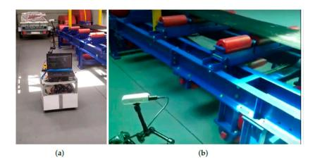
**Figure 17.** An inspection robot during the experiment: (**a**) general photo; (**b**) zoom on sensor (Reprinted from Ref. [109]).
