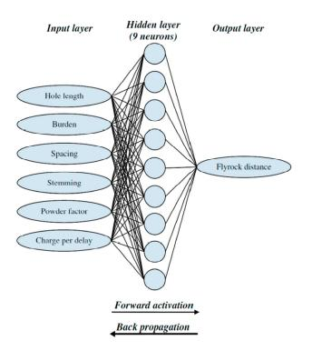
Figure 14. Architecture of artificial neural network in rock blasting (Reprinted from Ref. [93]).
