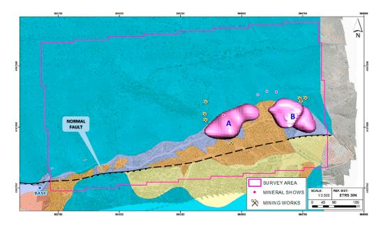
**Figure 20.** Three-dimensional model of the magnetic susceptibility of the Don Jacobo area, displaying the position of the two bodies of high magnetic susceptibility A and B; over the 1:5000 geological cartography and aerial RGB image of the area of Don Jacobo (Reprinted from Ref. [114]).
