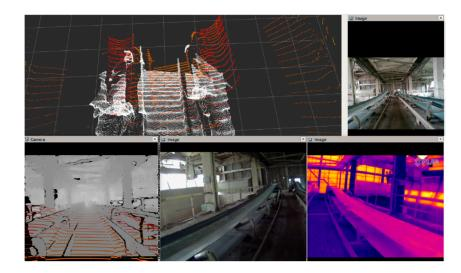
**Figure 18.** View in Rviz of recorded data during inspection. (**top left**): Depth camera data (gray) and lidar scan lines (red); (**top right**): Front overview; (**bottom left**): Depth camera data and lidar scan lines mapped onto 2D frontal view; (**bottom center**): RGB camera frame; (**bottom right**): IR camera frame (flipped horizontally) (Reprinted from Ref. [110]).
