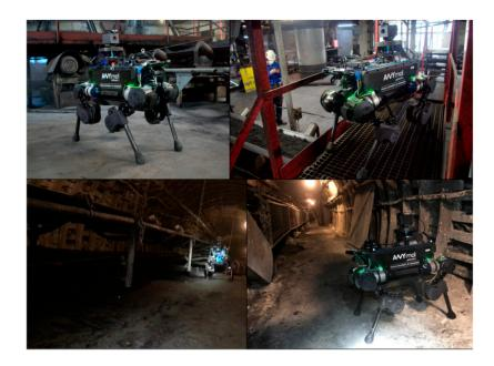
**Figure 19.** ANYmal legged robot by ANYbotics in various mining conditions (Reprinted from Ref. [111]).
