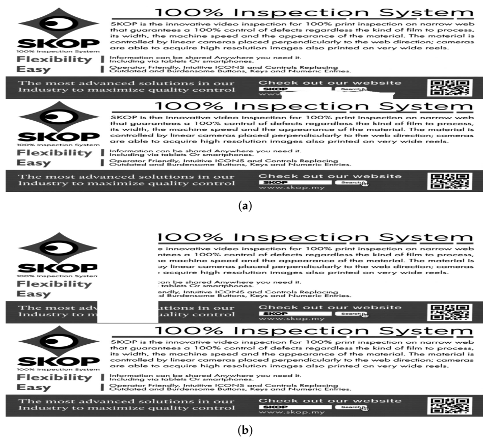
Figure 12. Aligned images. (a) Query image with small tampered area has been aligned with template image; (b) Query image with large tampered area has also been aligned with template image.
