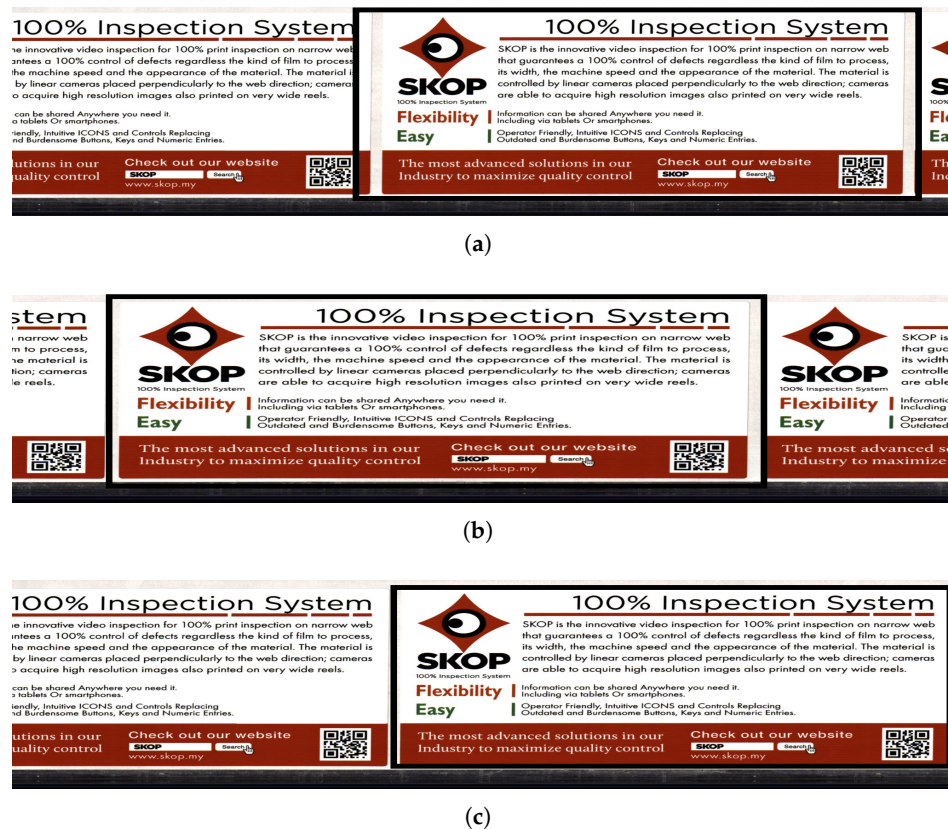
Figure 5. Images with background and marked ROI. (a) ROI is on the centre but left label has more area than right; (b) ROI is on the centre but right label has slight more area than left; (c) ROI is on the right side but on the left major portion of upcoming label is also present.
