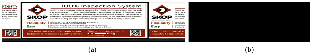
Figure 15. Correct label. (a) Query image with no fault; (b) Fully black mask indicates that the query image has no fault.
