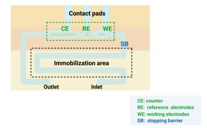
Figure 5. The structure of microfluidic chip.
