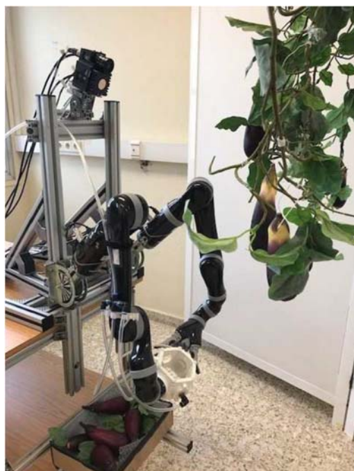
Figure 4. Soft gripper robotic arm designed in Spain for robotic agricultural harvesters [8].
