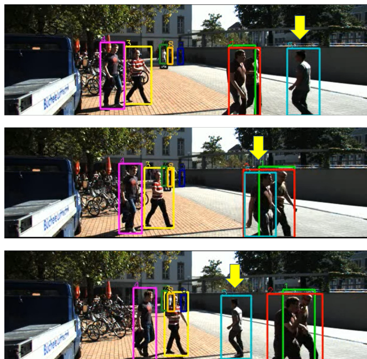
Figure 2. Preserving the ID during full occlusion. The frames are obtained from the MOT15 dataset [19]. The yellow arrow is pointing towards a track ( top image ) that experiences full occlusion ( middle image ). The objective of the MOT system is to preserve the ID of the track ( bottom image ) and matches the previously detected object with the reappeared one.
