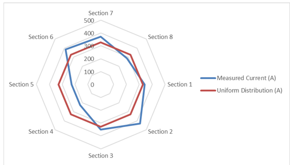
Figure 4. The measured distribution of the electrode current within the section feeders (blue line) and the desired uniform distribution (red line), with reference to the nominal current (2625 A).
