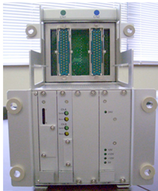
Figure 10. Control unit for the Bogie Abnormal Swing Detection System.
