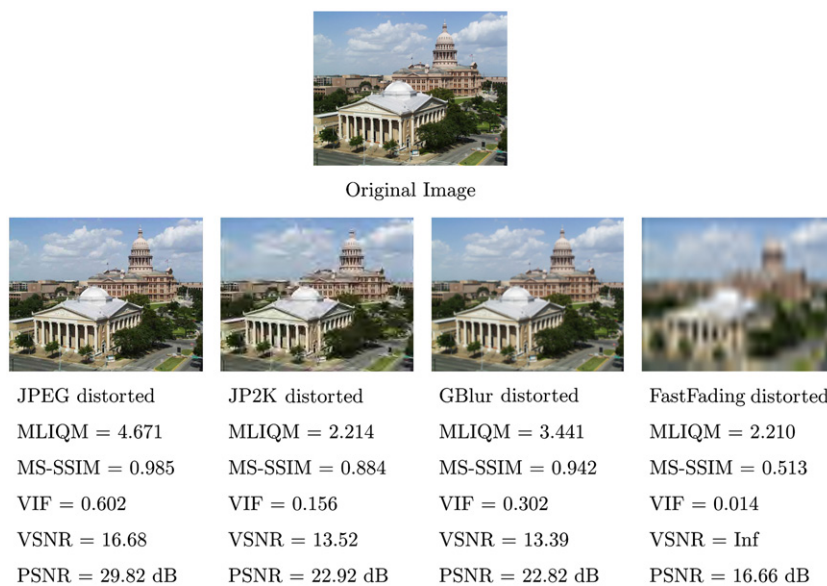
Fig. 4. Example of results obtained computing the trial FR-IQA algorithms on an original image (churchandcapitol extracted from LIVE and its degraded versions by applying JPEG (0.83865 bpp), JPEG2000 (0.194 bpp), Gaussian blur ( \sigma = 1.565074 ) and a fast fading process (receiver SNR=18.9).
