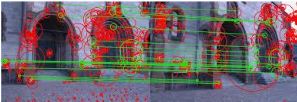
Figure - 2: Comparison between the two Images using Keypoints for Image match using SIFT Feature
