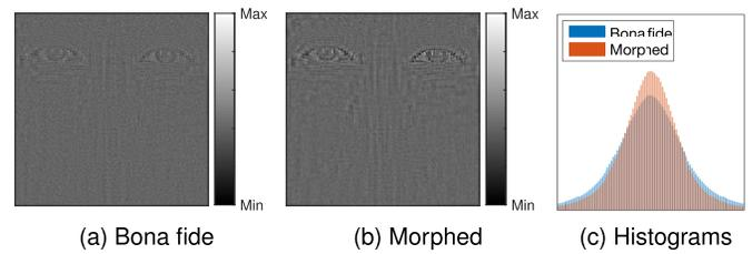
Fig. 3. PRNU values and histograms of the PRNU extracted from a single bona fide image (a) and morphed face images (b). The PRNU values have been averaged over 500 randomly selected images of the FRGCv2 dataset.
