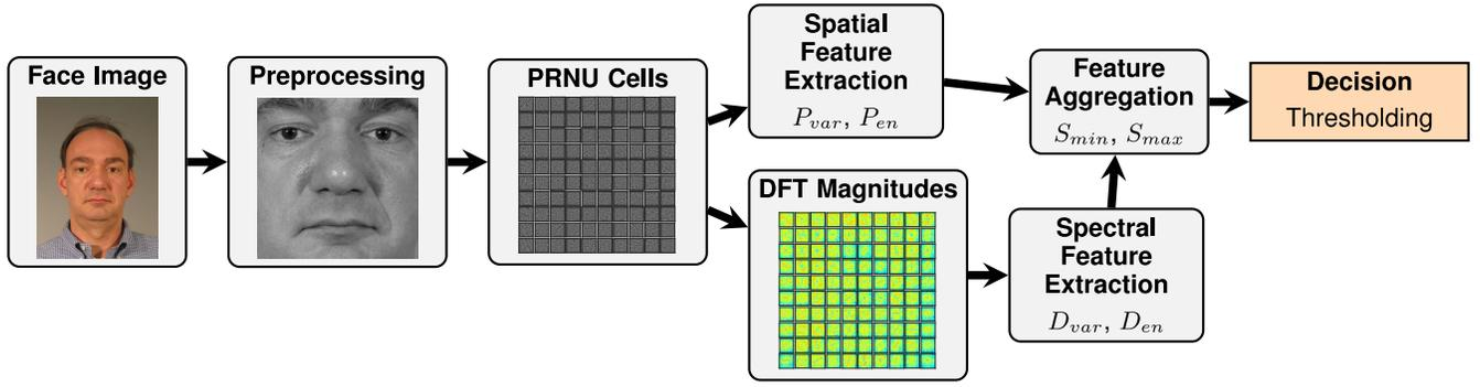
Fig. 5. Processing steps of the proposed PRNU-based morph detection system and different feature types: spatial features (upper path) and spectral features (lower path).
