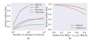
Fig. 4. (a) Comparison of sampling efficiency. With only 1/10 samples, SABLAS achieves a nearly perfect relative safety rate. (b) Influence of model error on safety performance. SABLAS- $\mathcal{L}_{p2}$  uses (6) instead of the proposed (7) as loss function. SABLAS is tolerant to large error between nominal and real models while keeping a high safety rate.
