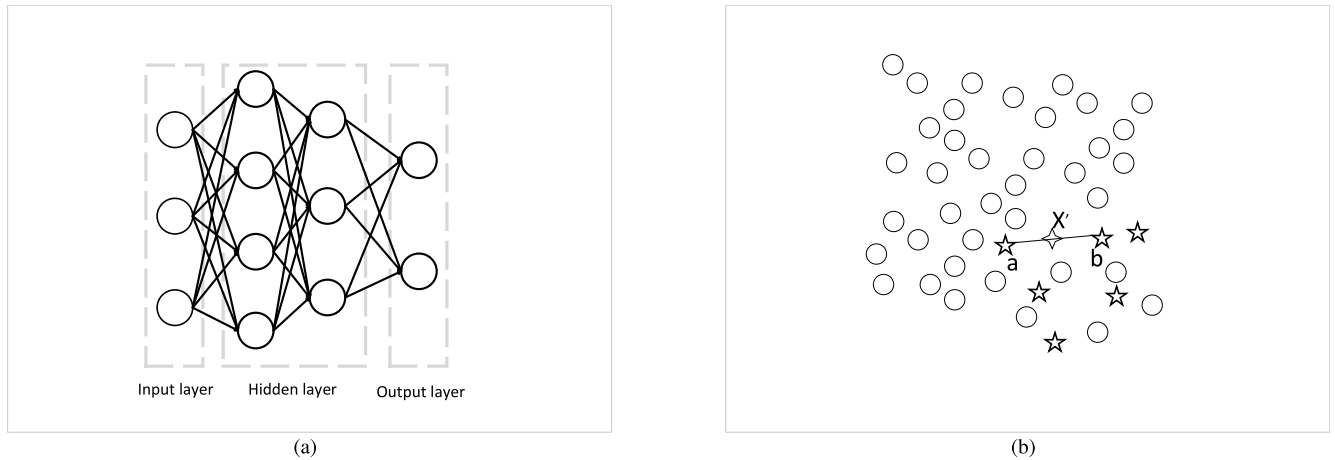
FIGURE 1. (a):The pre-processed data flows into the hidden layer of the neural network, then the features of the input data are abstracted at multiple levels in the hidden layer,so that the output result supports the clearest classification by the classifier. (b):The new sample x' generated by the SMOTE method is any point on the line connecting the minority samples a and b , where sample a is randomly determined, and sample b is the nearest neighbor sample of sample a .
