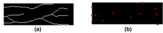
FIGURE 7. Minutiae pattern extraction: (a) skeleton image; (c) minutiae patterns from (a), which are marked in red color.
