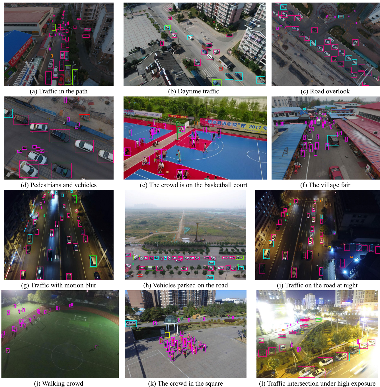
FIGURE 13. The detection results of VisDrone2019 dataset.
