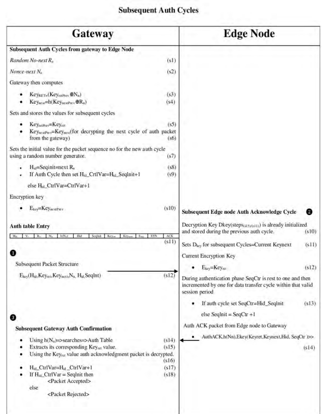
FIGURE 2. A high-level summary of the subsequent authentication cycle.
